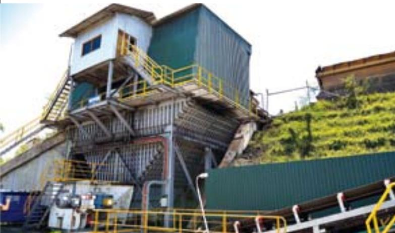
Each single conveyor at Kelanis can load up to 2,000 tonnes per hour on to waiting barges.
